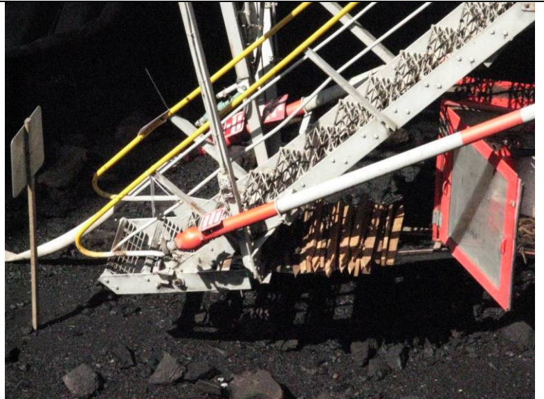
Photo#68 Showing rotary hose connection and the birds mouth connection on the other side
