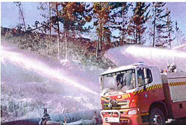
Pictured above: Compressed Air Foam System Truck from Tasmania is concentrating its efforts on fire suppression on the Northern batters.
