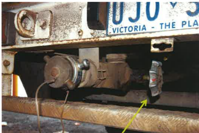
Open valve to fill tank
