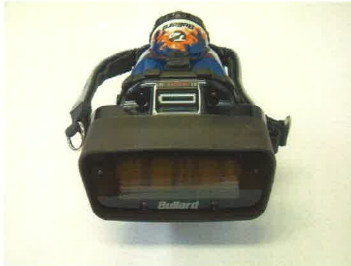
Thermal Imaging Camera
