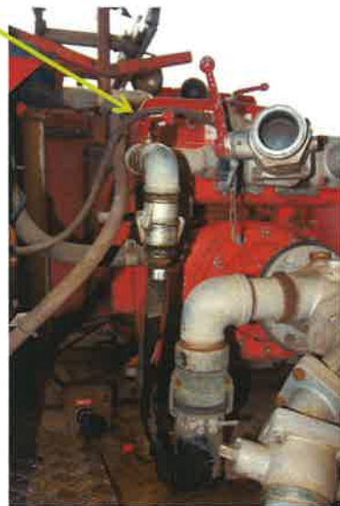
This valve turns on the live hose reel
