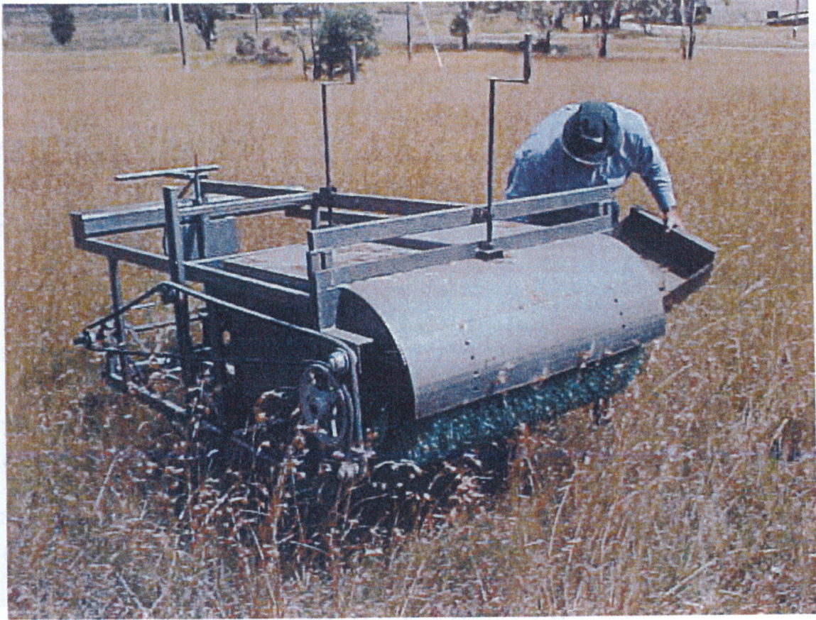
Mechanical Harvesting of Kangaroo Grass ( Themeda triandra ) seed from the 'Ridge Reserve' for revegetation works (Alliance Seeds P/L).
