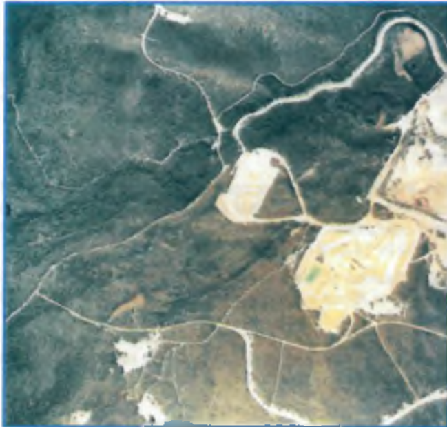
Plate 1c: In 1998, the landscaping portion of the rehabilitation is completed on No.2 pit with a layer of topsoil and contour ripping
