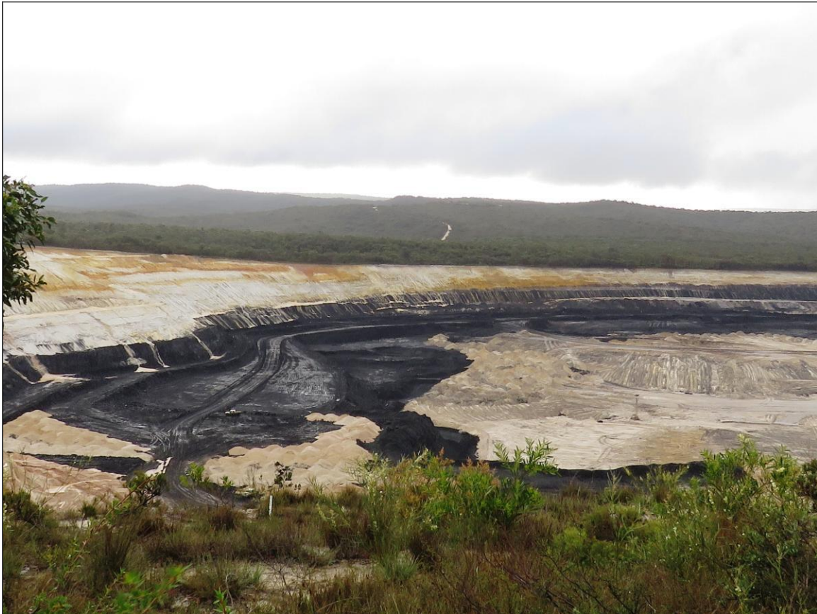
Figure Eight: The coal face on the western wall of the mine will not be covered with overburden
