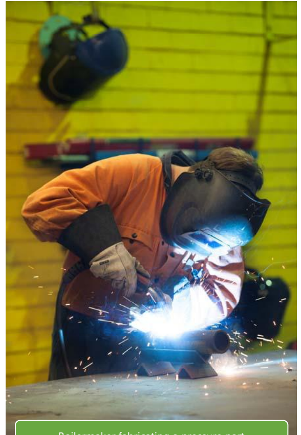
Boilermaker fabricating a pressure part
