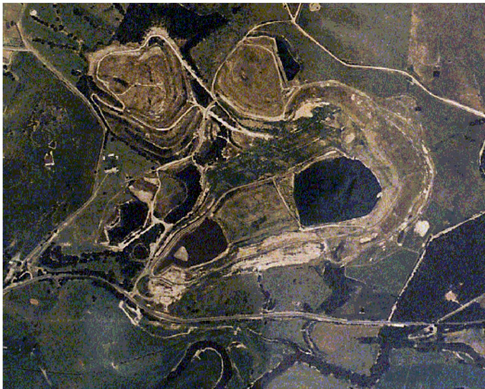
Figure 7 An aerial view of the YNEOC lake system circa 1995 prior to rehabilitation works of the overburden dumps and surrounding areas having been completed. The large mid-field overburden dump and the small overburden capped island in the southern lake are clearly visible.
