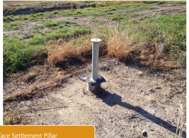
Surface Settlement Pillar
