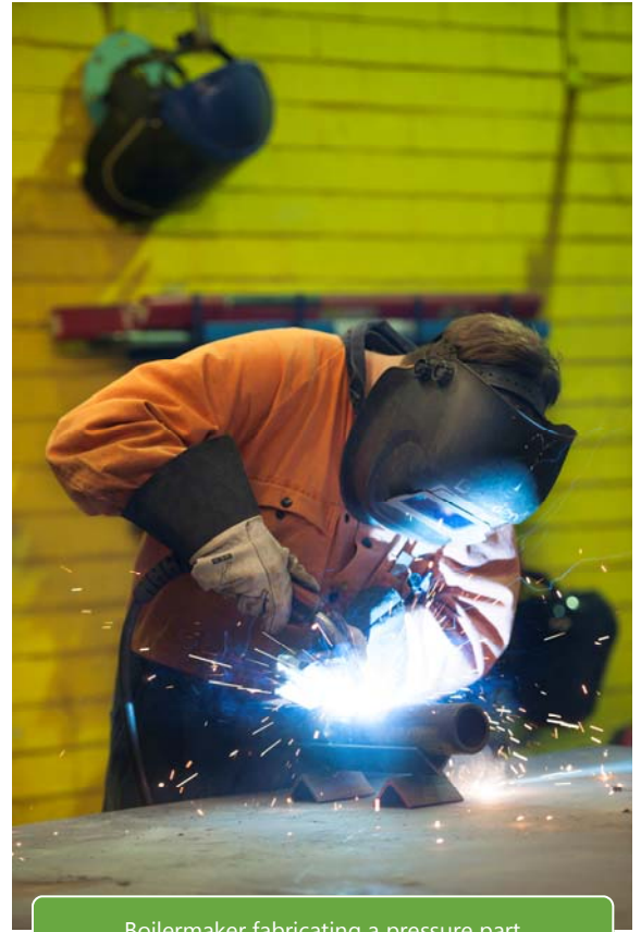
Boilermaker fabricating a pressure part
