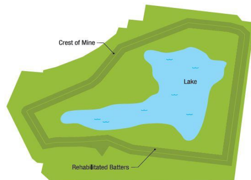
PARTIAL BACKFILL BELOW THE WATER TABLE
