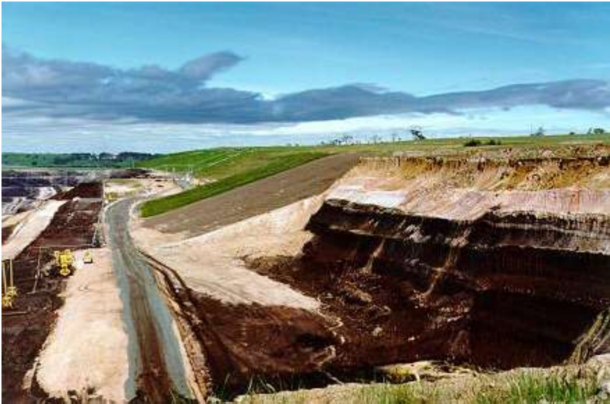
Figure 3 Upper Mine Batter Rehabilitation Trials
